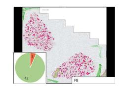
**Figure 1.** Color-phase SEM images of K feldspar grains (pink). Grain sizes increase left to right, and pie charts show number of grains where Pb isotope ratios are >0.5% (green) or <0.5% (red) based on lolite data reduction post-laser ablation.
